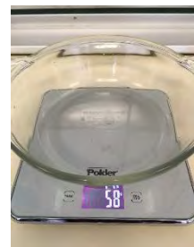
Weight of water displaced (the weight of the glass bowl was tared (or zeroed)).
